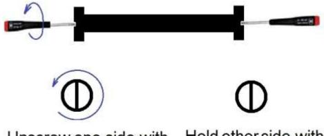
Unscrew one side with a slot Screwdriver
